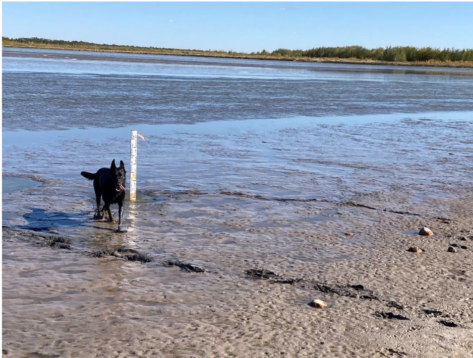
Staff gauge at Plover Pt. SCL Park el. 733.8m (Record low Sept 2022)
